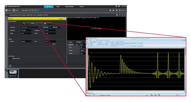
Figure 1. Design and build arbitrary waveform with Benchlink Waveform Builder Pro within BenchVue Function Generator App.
