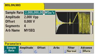
Waveform generator display of the desired sequence.
