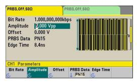
Test your digital serial buses by streaming standard PRBS patterns—PN3 through PN32.
